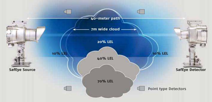
This scenario shows how the matrix of point type detectors can miss a leak or eventually only see diluted gas levels whereas SafEye 700 Open-Path will, in this case, measure 20% LEL x 7 m = 1.4 LEL.m - well above 1 LEL.m alarm level
